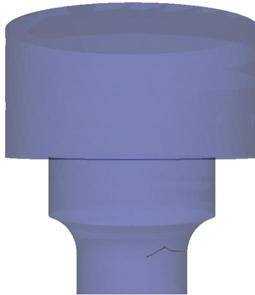
Figure 64 – Crack growth path followed by the tip of the main crack predicted for specimen 1383-16 (EDF weld registered RND-M-D-1054). Code\_Coriolis prediction relying on the index model and the sigmoid growth law. Detailed view at the head/shank junction.
