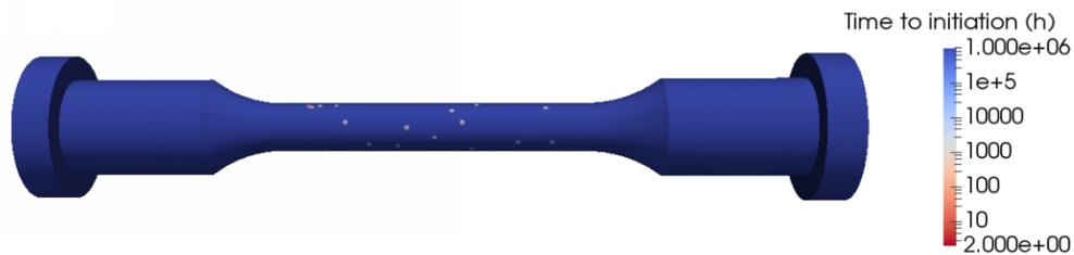
Figure 105 – Time to initiation field predicted for specimen 1383-01T (EDF weld registered RND-M-D-711). Code\_Coriolis prediction relying on the local model and the sigmoid growth law.
