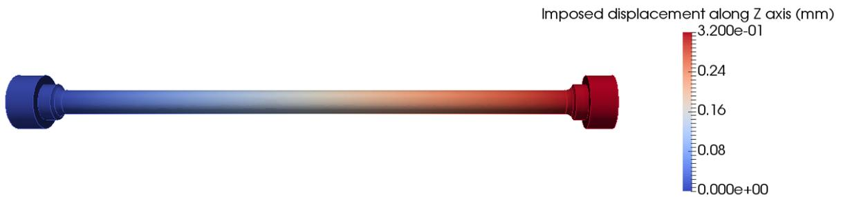
Figure 52 – Displacement field imposed on the TL2-type specimen #1383-11.
