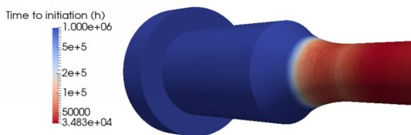
Figure 71 – Time to initiation field predicted for specimen 1383-01T (EDF weld registered RND-M-D-711). Code\_Coriolis prediction relying on the index model and the sigmoid growth law. Detailed view at the head/shank junction.
