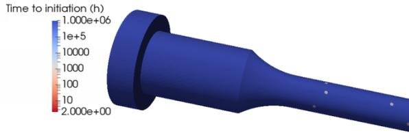
Figure 106 – Time to initiation field predicted for specimen 1383-01T (EDF weld registered RND-M-D-711). Code\_Coriolis prediction relying on the local model and the sigmoid growth law. Detailed view at the head/shank junction.
