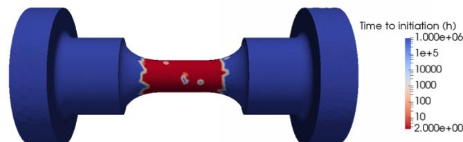
Figure 122 – Time to initiation field predicted for specimen IN194 (PNNL weld registered KAPL 823030). Code\_Coriolis prediction relying on the local model and the sigmoid growth law.
