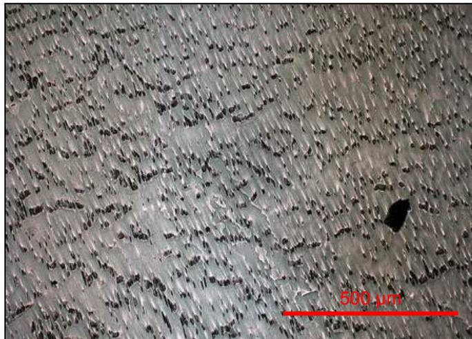
Figure 8 – Microstructure of Alloy 82 registered as RND-M-D-711.
