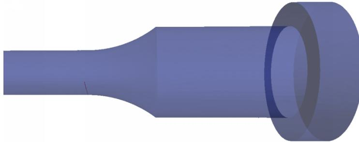
Figure 108 – Crack growth path followed by the tip of the main crack predicted for specimen 1383-01T (EDF weld registered RND-M-D-711). Code\_Coriolis prediction relying on the local model and the sigmoid growth law. Detailed view at the head/shank junction.
