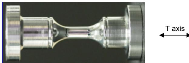
Figure 29 – PNNL-type specimen.
