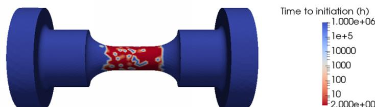
Figure 113 – Time to initiation field predicted for specimen IN171 (PNNL weld registered Studsvik 8001231). Code\_Coriolis prediction relying on the local model and the sigmoid growth law.
