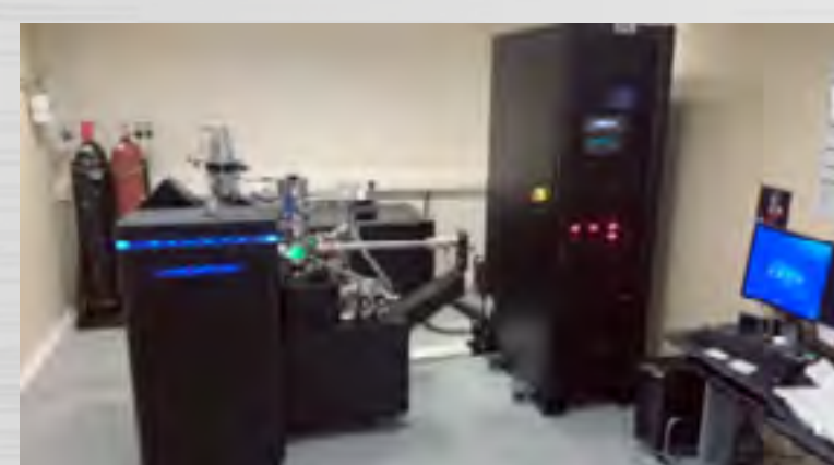
Kurchatov Institut : Atom probe tomograph Cameca LEAP 4000 HR
